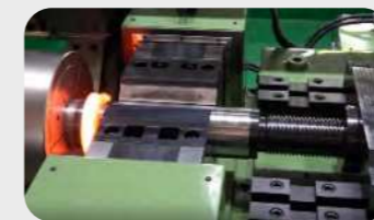
4. Sudden stop of SPINDLE, UP SET pressurization
