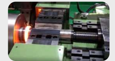
3. Start contacting with materials, friction heating
