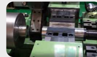
1. Fix welding materials to the side of SPINDLE and TABLE side
