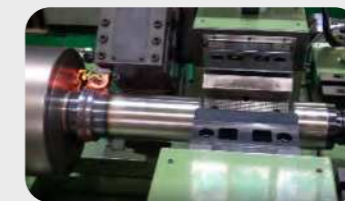
5. Cut uplifted parts made when heating pressurization
